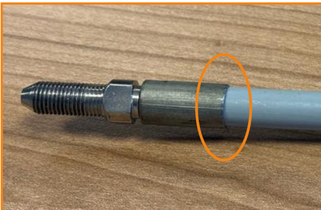
Typical “Blast-Pro” crimp fitting that could pass through the hose catcher
