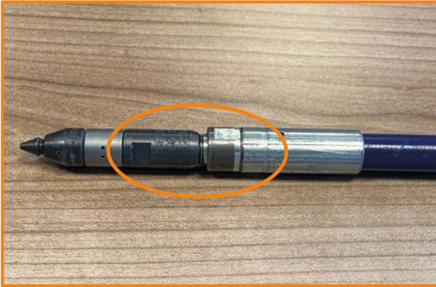
Nozzle diameter smaller than crimp fitting diameter = incorrect
