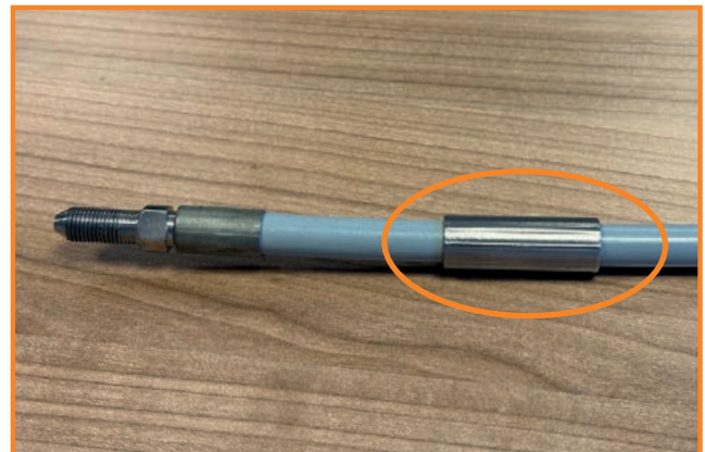
Always use a stop sleeve when using “Blast-Pro” or “Pro-Lance” crimp fitting
