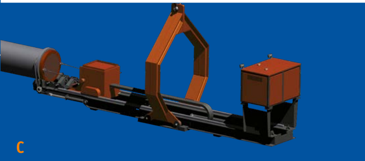
Connect pulling slings of the pull car to tube sheet
