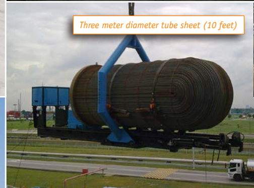
100T bundle puller with 100T winch capacity
