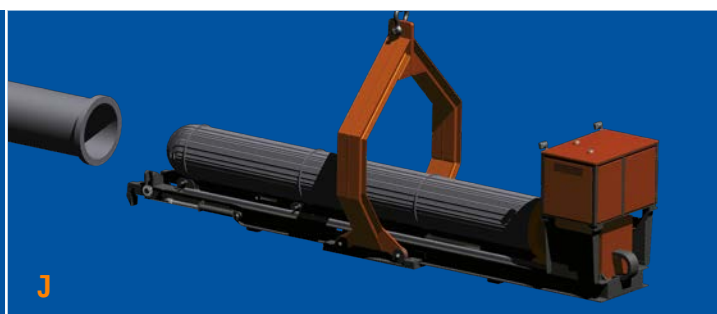
When slings are loose, disconnect and remove extractor
