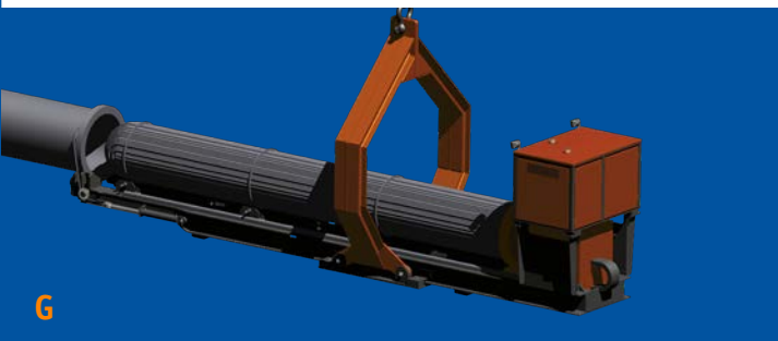
Pull out bundle completely
