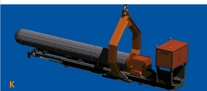
Position extractor on the ground and move lifting frame backwards to remove bundle
