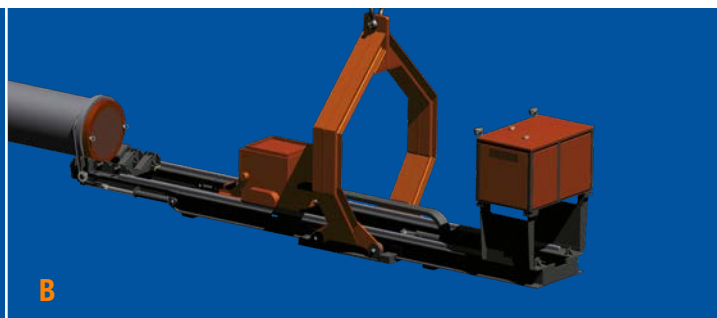
Connect slings to shell flange and clamps behind shell flange
